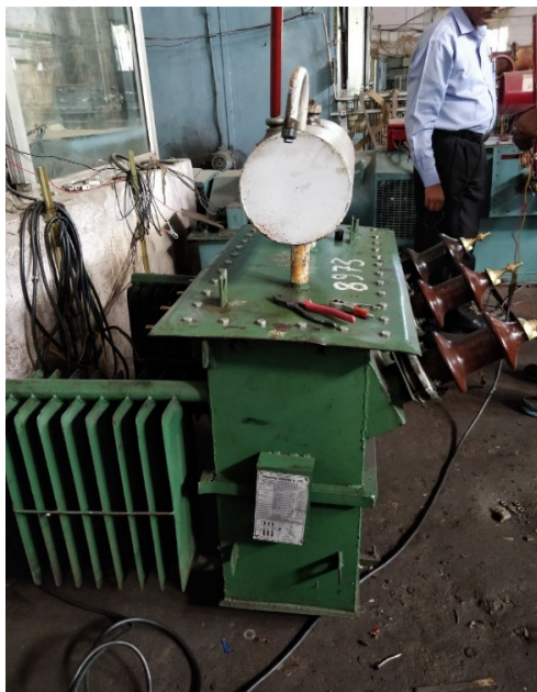
Figure 7. Tank Placement on assembled DT
