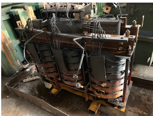
Figure 13. Acquired failed DT
