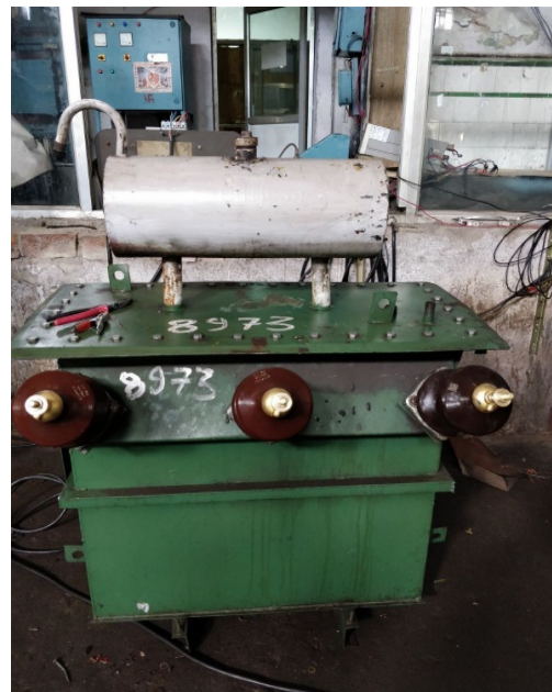
Figure 8. Final repaired DT
