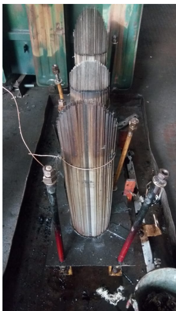
Figure 15. Acquired failed DT core
